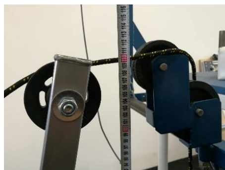
Figure 1. Incorrectly set calibration height during initial testing of AB EX
